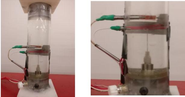
Figure 2. Details of instrumentation of polycarbonate cylinder used in testing of bubble collapse under shock wave loading: the location of two Kulite pressure sensors, strain gages and air delivery port with 27 gauge needle are illustrated.
