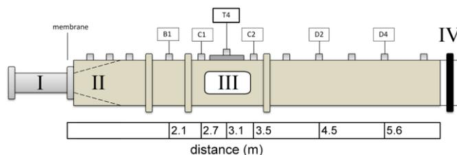
Figure 1. The 9 inch diameter square cross section shock tube schematics illustrating the location of pressure sensors (B1 to D4) employed to measure incident shock wave characteristics. The design of the shock tube consists of four components: the breach (I), the expansion section (II), the test section (III) and the end plate (IV) [5].
