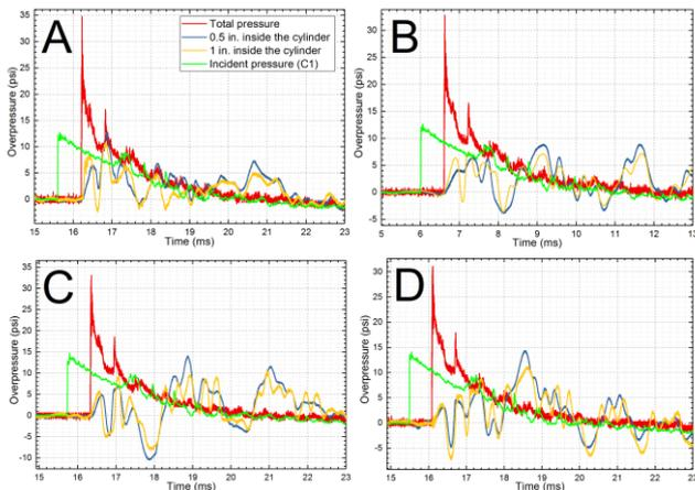
Figure 3. Pressure-time profiles recorded by incident (C1), total (on the front surface of the cylinder) and fluid (inside the cylinder) sensors: A) deionized water without bubbles, B) 50% glycerol in water solution without bubbles, C) deionized water with bubbles, D) 50% glycerol in water solution with bubbles.
