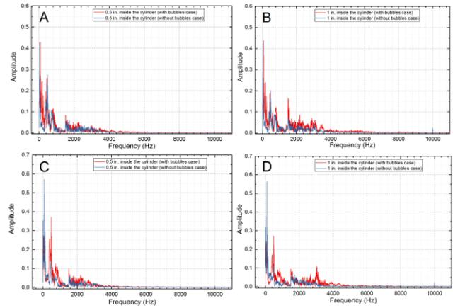
Figure 4. The effect of air bubbles on frequency of pressure histories reported by sensors immersed in: A) glycerol (bottom sensor: 0.5 in. inside), B) glycerol (top sensor: 1 in. inside), C) water (bottom sensor: 0.5 in. inside) and D) water (top sensor 1 in. inside).
