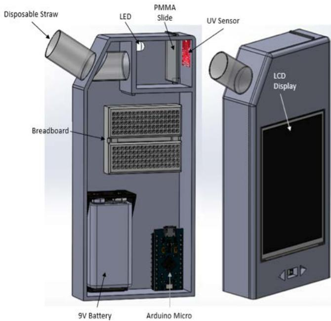
Fig. 1: Final proposed concept for the diabetic breathalyzer.
