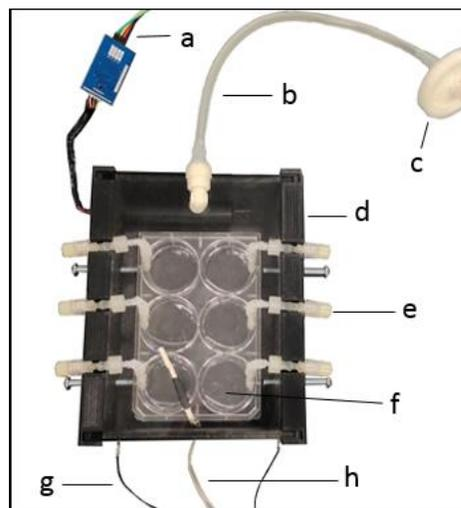
**Figure 1:** Device design: a) CO<sub>2</sub> sensor interface, b) CO<sub>2</sub> input tubing, c) CO<sub>2</sub> in-line filter, d) device holder, e) perfusion inputs, f) modified 6-well plate cover, g) transparent heater (under device) wires, and h) thermistor wire.
