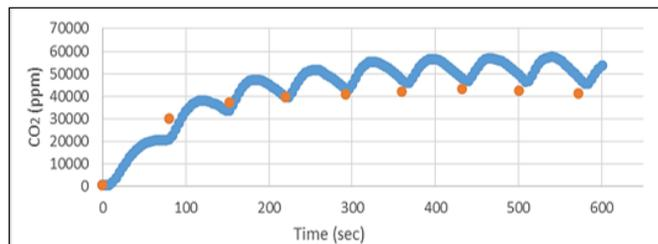
Figure 3: CO<sub>2</sub> sensor measurements (blue) and Vernier sensor (orange) with control system over time, measured in parts per million (ppm)
