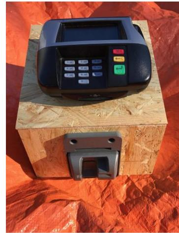
Fig. 3. Fully constructed test stand with card readers.
