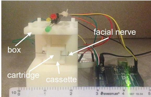
Fig. 2. Components of simulation model with the cartridge containing the ossicular chain (not visible). The cassette positions the cartridge and facial nerve. The box interfaces with the exterior shell and contains the force sensor (not visible) under the cassette. On the right side, Arduino and breadboard will be installed with the model and connected to LEDs.
