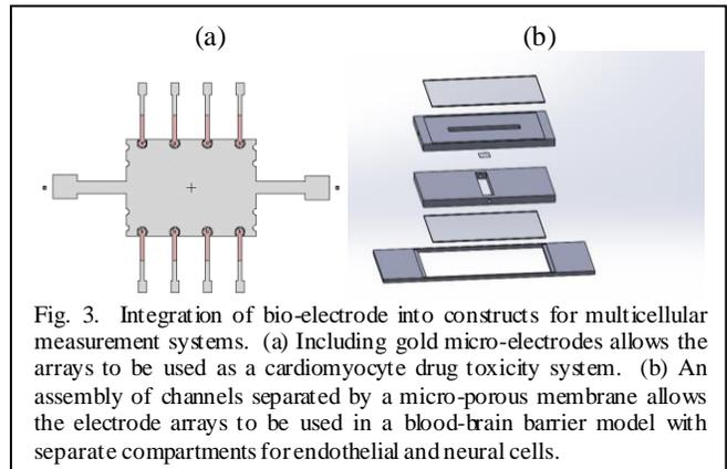
Fig. 3. Integration of bio-electrode into constructs for multicellular measurement systems. (a) Including gold micro-electrodes allows the arrays to be used as a cardiomyocyte drug toxicity system. (b) An assembly of channels separated by a micro-porous membrane allows the electrode arrays to be used in a blood-brain barrier model with separate compartments for endothelial and neural cells.
