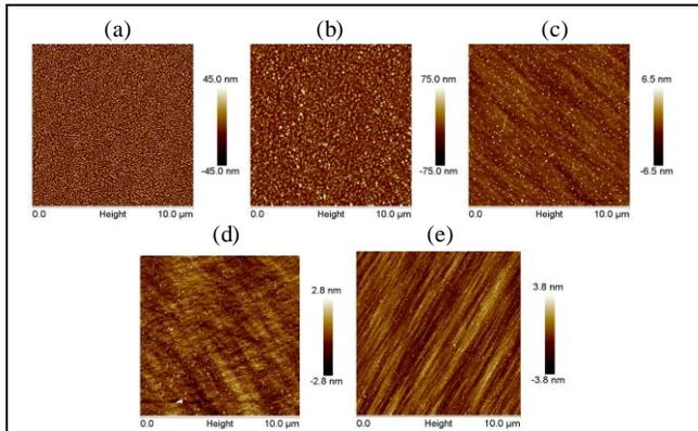
Fig. 1. Representative AFM images of ITO sputtered fused silica surfaces with plasma oxygen concentrations at (a) 0%, (b) 2.5%, (c) 5.0%, (d) 7.5%, and (e) 10%. Increasing the plasma O<sub>2</sub> concentration from 0 to 10% tends to produce smoother surfaces.
