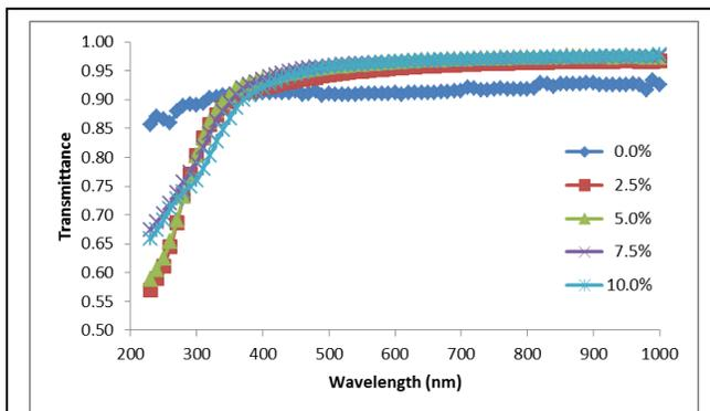
Fig. 2. Optical absorption spectra of ITO coated fused silica wafers with varying sputter oxygen feed concentrations. Increasing the oxygen plasma concentration increases the transmittance above 400nm. Below 300 nm increasing oxygen concentrations decrease the transmittance.
