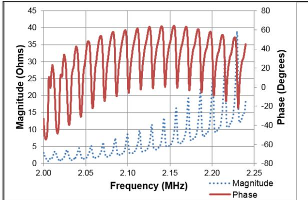
Fig. 2. Impedance spectra of a 2MHz PZT-8 transducer. The observed resonance peaks with the attached transducer were used to determine the driving frequency. During the measurement the chamber was filled with water.
