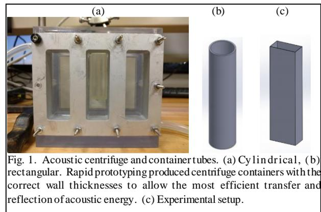
Fig. 1. Acoustic centrifuge and container tubes. (a) Cylindrical, (b) rectangular. Rapid prototyping produced centrifuge containers with the correct wall thicknesses to allow the most efficient transfer and reflection of acoustic energy. (c) Experimental setup.
