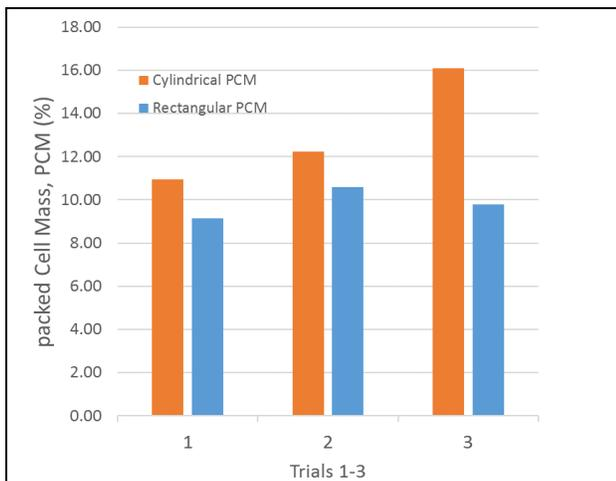
Fig. 3. The Percentage pack cell mass remaining in the supernatant following acoustic centrifugation using cylindrical and rectangular centrifuge containers. The value of p value is
