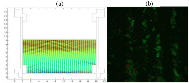
Fig. 3. Computer simulation and microscopy image of non-adherent cancer cell clusters. (a) The standing waves produced within the bioreactor were a function of both the bioreactor dimensions and fluid height. (b) Well defined cancer cell clusters are produced within the acoustic fields. Viable cells are stained green and dead cells orange.
