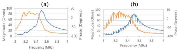
Fig. 2. Impedance spectra of acoustic bioreactor chamber half-filled and completely filled. (a) The impedance spectra with the chamber half-filled showed well defined anti-resonance peaks. (b) With the chamber completely filled a series of additional resonance and anti-resonance peaks were observed.
