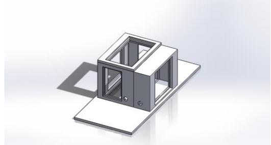
Fig. 1. Acoustic bioreactor. A PZT-8 transducer driven at 3Mz produced standing acoustic waves within the bioreactor for trapping cells. A cooling chamber next to the transducer prevented heat generation from destabilizing the bioreactor.
