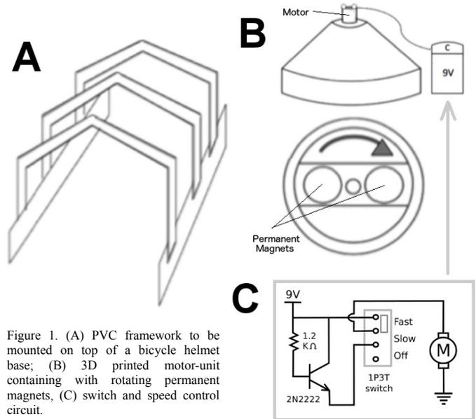
Figure 1. (A) PVC framework to be mounted on top of a bicycle helmet base; (B) 3D printed motor-unit containing with rotating permanent magnets; (C) switch and speed control circuit.
