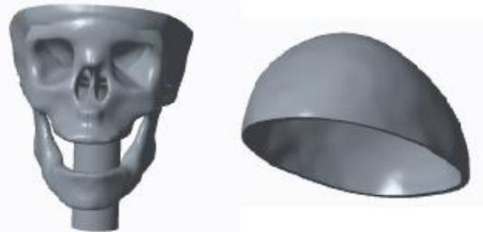
**Figure 1: CAD model of skull courtesy of ARL. This model was originally an aggregate of hundreds of MRI scans from soldiers, later converted to a CAD file for printing.**
