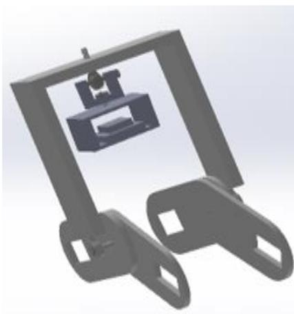
Fig. 1. PatFinder device with gyroscopes enclosed.
