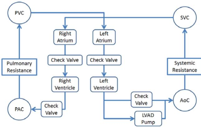
Fig. 2. Diagram of mock circulatory loop assembly
