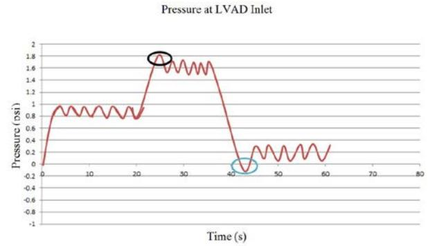
Fig. 3. Pressure at the inlet of LVAD pump
