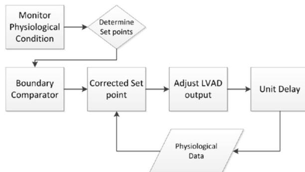
Fig. 1. Control system logic flow
